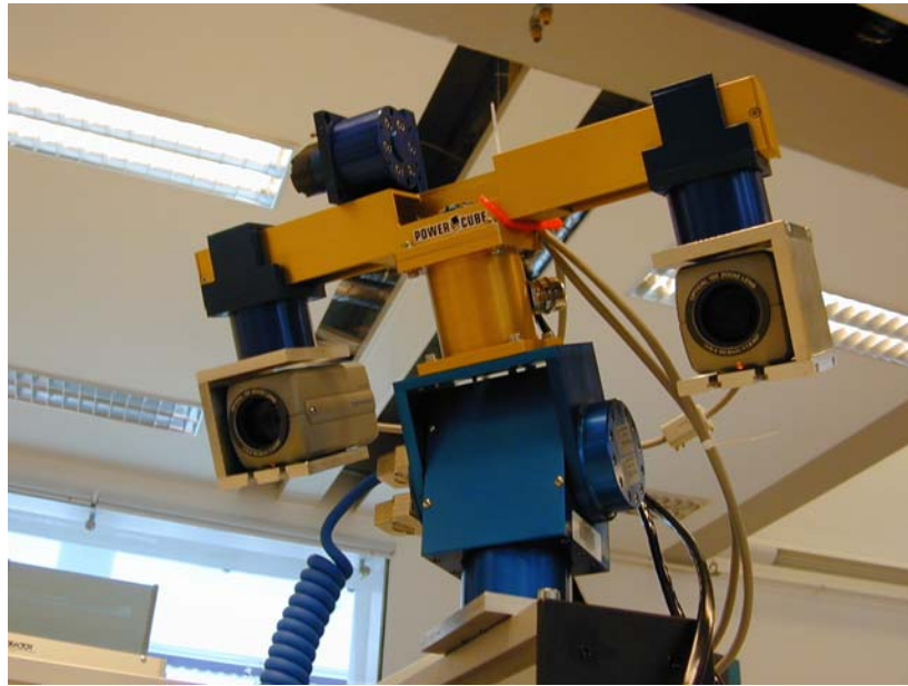
Figure 1: The stereoscopic head (courtesy Profactor GmbH) that is used to acquire image stereo-pairs that feed the HT component.
