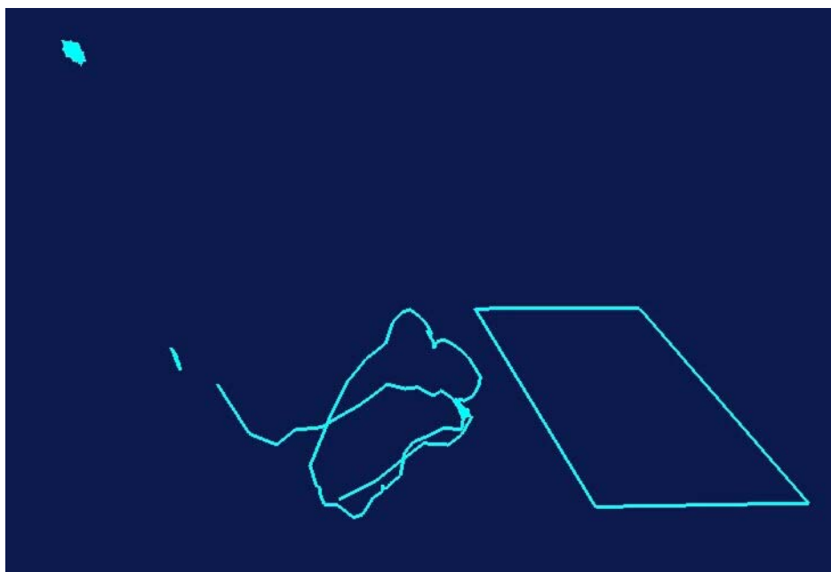
Figure 8: The 3D trajectories of the hand hypotheses detected in the experiment of Fig. 6. The top-left and middle-left isolated spots correspond to the motion of the operator's head and of the arm of the armchair, respectively. The trajectory in the center of the image corresponds to the hand trajectory. The upper facet of the CD player has also been reconstructed, as a reference.
