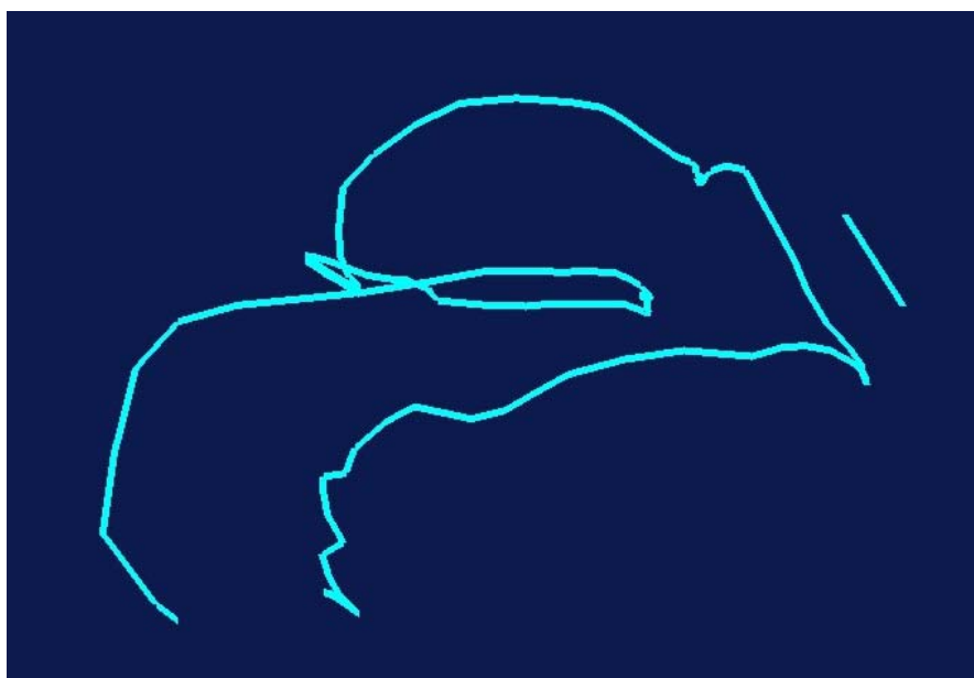
Figure 9: The 3D trajectories of the hand hypotheses detected in the experiment of Fig. 7. The straight line segment appearing in the right part of the figure corresponds to the tray of the CD player.
