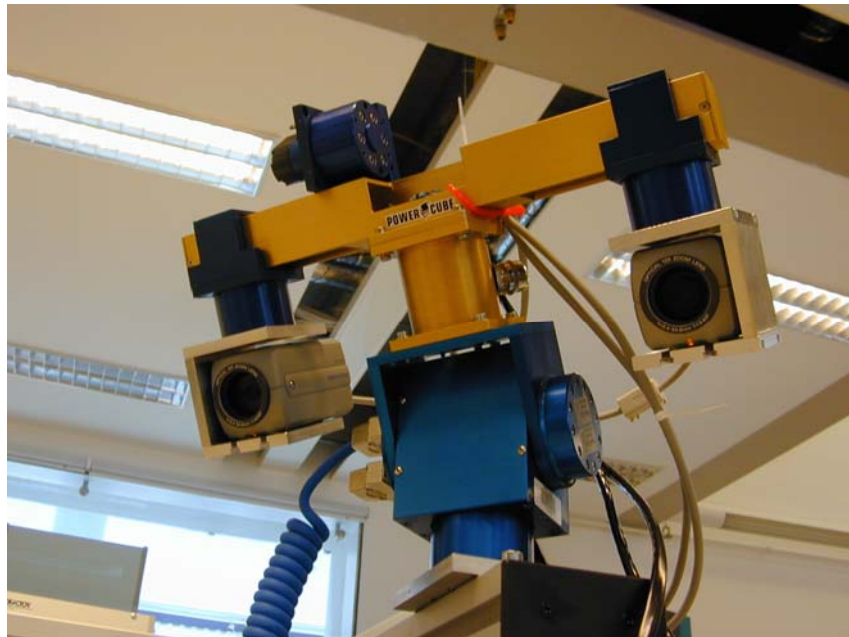
Figure 1: The stereoscopic head (courtesy Profactor GmbH) that is used to acquire stereo image pairs that are fed to the developed SCRT system.
