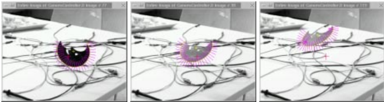
Figure 6: Samples of tracking an ellipse arc. The ellipse tracked is displayed in yellow.
